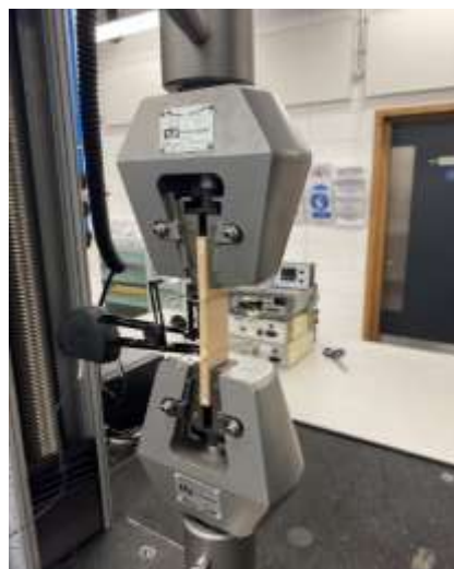
Figure 4: Tensile testing of wood specimen.
