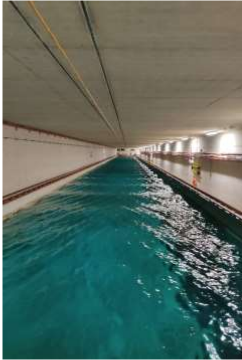
Figure 5: Picture looking down the towing tank from the carriage showing the waves.
