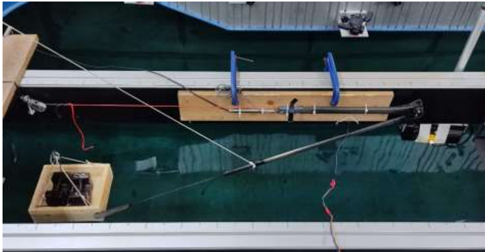
Figure 6: Experimental setup on the carriage showing wand system, sensor, and weights.
