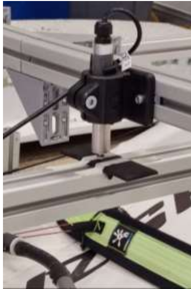
Figure 3: LDIV testing on the deflection of wing bars.
