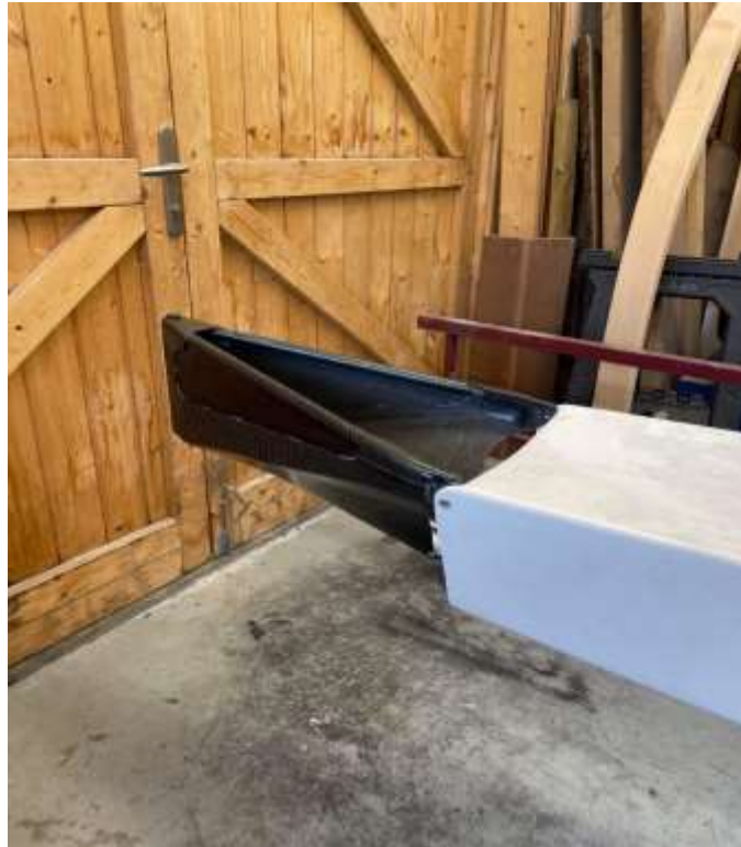
Figure 7: Picture showing the gantry fixed onto the stern of the boat.
