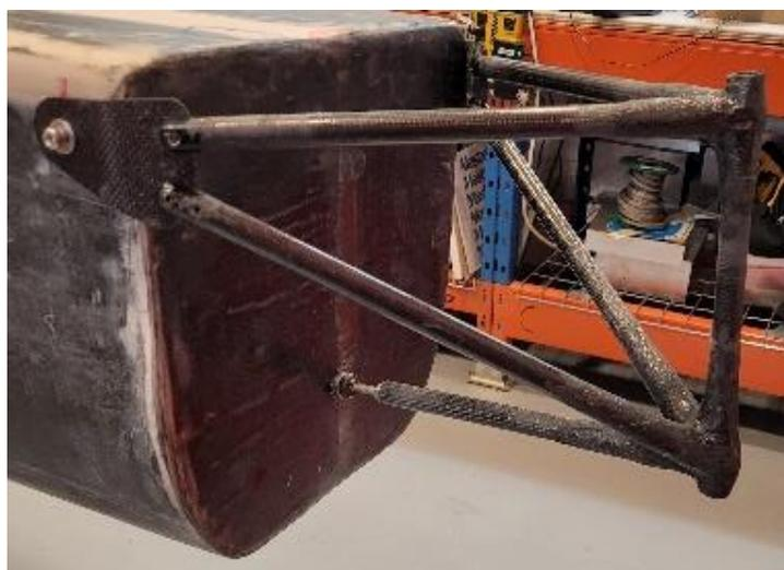
Figure 9: The finished rudder structure
