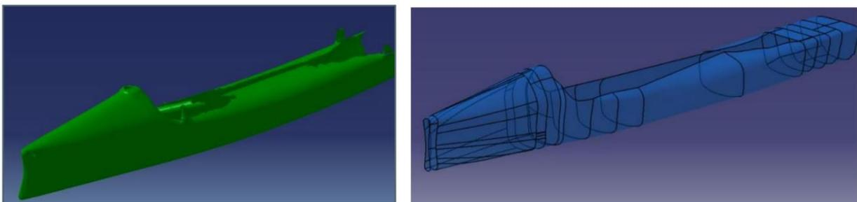
*Figure 1: Scanned Waszp hull, point cloud (left) and CAD model (right)*
