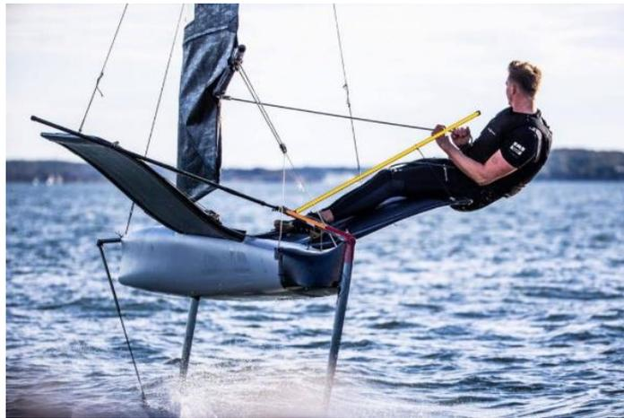
Figure 13: Moth under sail showing the tiller assembly
