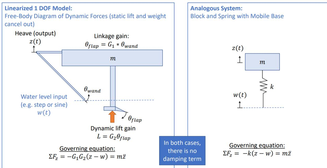
Figure 12. Single DOF model of the wand's effect on ride height
