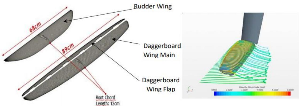
Figure 7 : Wing design embodiment (left) and CFD streamline visualization (right).
