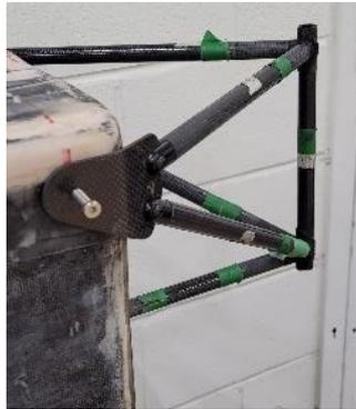
*Figure 26: Rudder structure being assembled on the transom*
