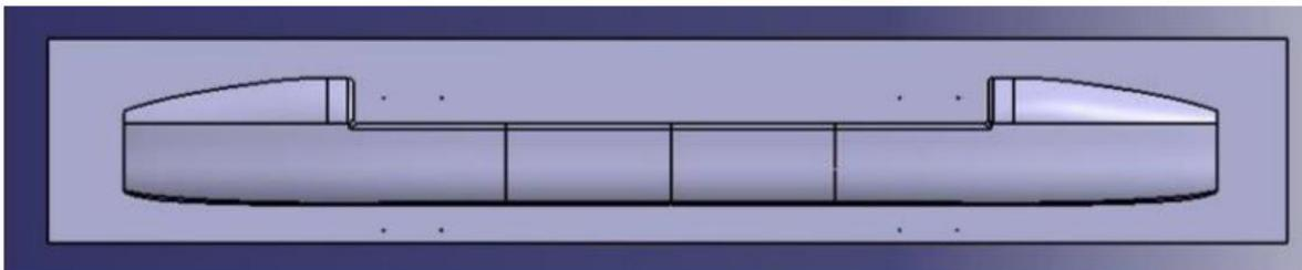
Figure 2: Symmetrical mould for making Rafale 3's hull.
