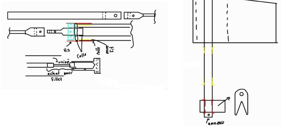
Figure 14: Tiller assembly schematics
