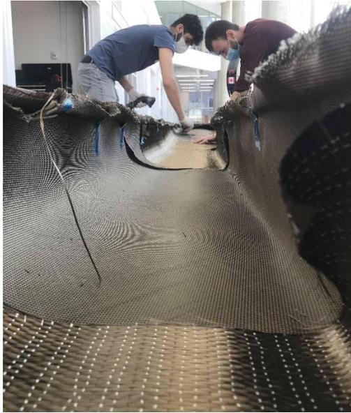
Figure 19: Lamination process of dry basalt fibre
