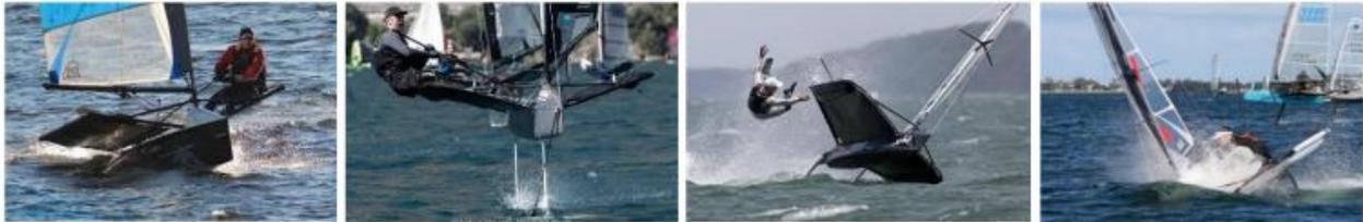
Figure 5 : Left to right: takeoff, steady flight, capsize and nosedive.
