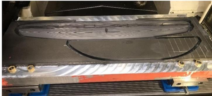
Figure 23: Clamped slab with contoured rudder wing (bottom) and surfaced daggerboard wing (top)
