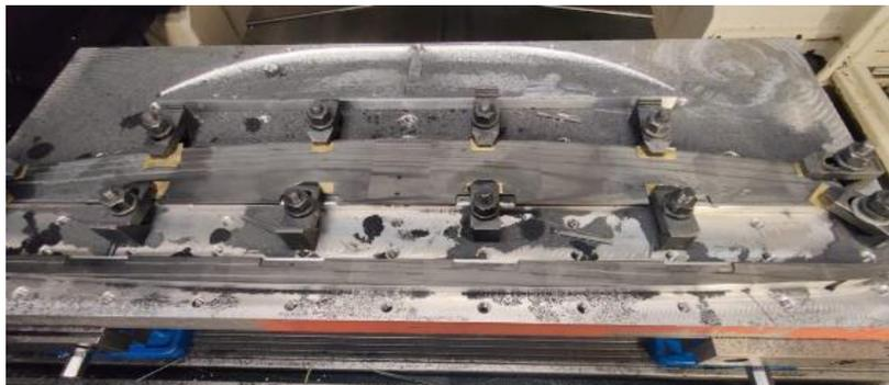
Figure 24: Aluminum work-holding jig with the main daggerboard wing mounted using step clamps
