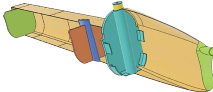
*Figure 4: Bulkhead positioned in the hull to reinforce zones of high loads.*
