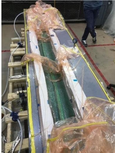
*Figure 21: Elium resin being injected into the starboard hull shell*
