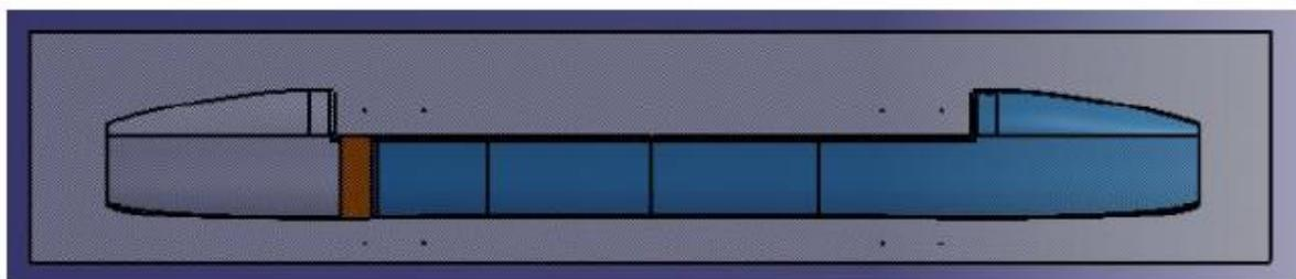
Figure 3: Port hull shell as made inside of the symmetrical mould.
