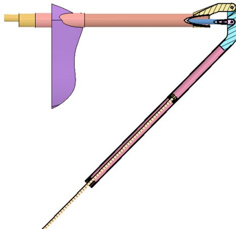
Figure 10. Cross-section of wand showing telescoping mechanism.
