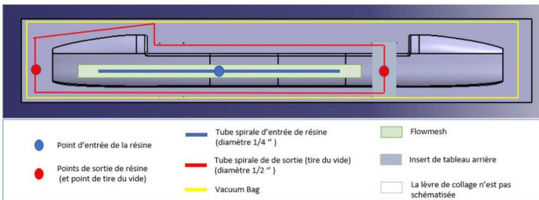
Figure 20: Schematic of the infusion process of the starboard hull shell
