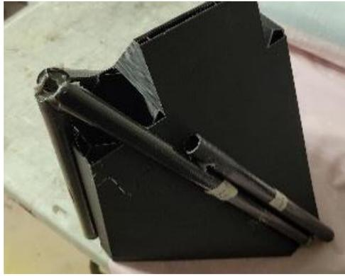
*Figure 25: Rudder structure being assembled on its jig*
