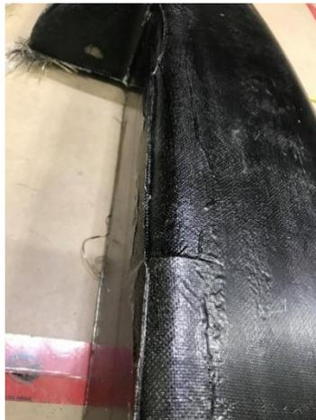
*Figure 22: Surface waviness resulting from inadequate fibre compaction*
