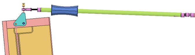
Figure 11. Wand bell crank with adjustable gearing and horizontal pushrod with adjustable rod end.
