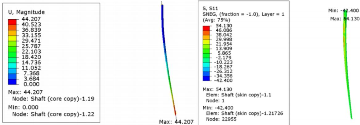
Figure 8 : Sample FEA results for tip deflection and root stress
