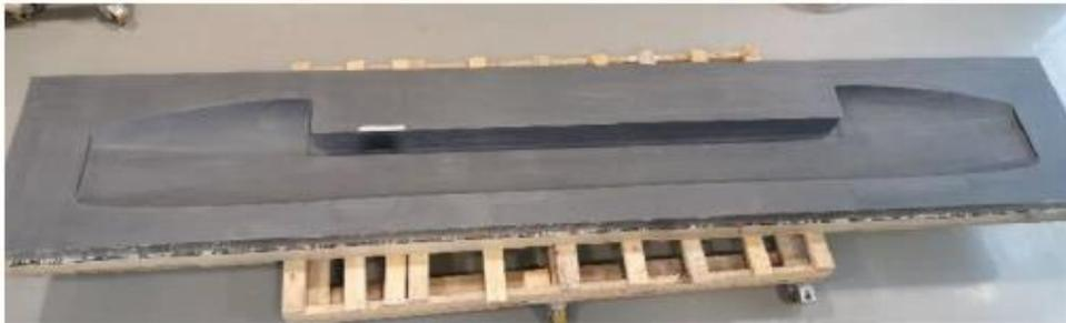
Figure 16: Symmetrical pinewood mould coated with Duratec
