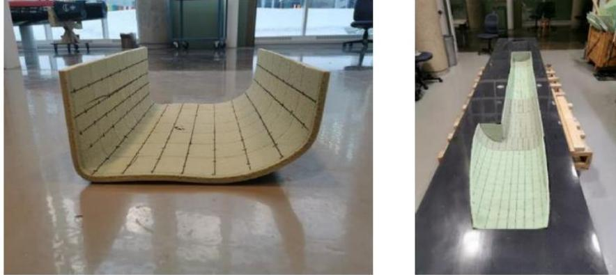
Figure 18: Thermoformed hull core sheets
