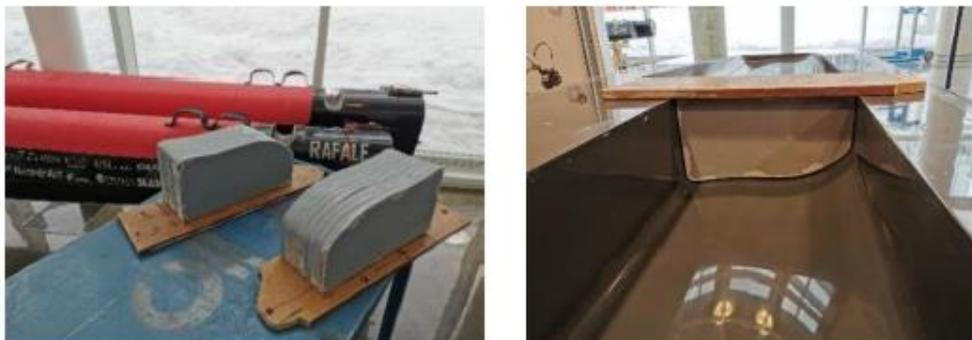
Figure 17: Mould inserts for making the transom
