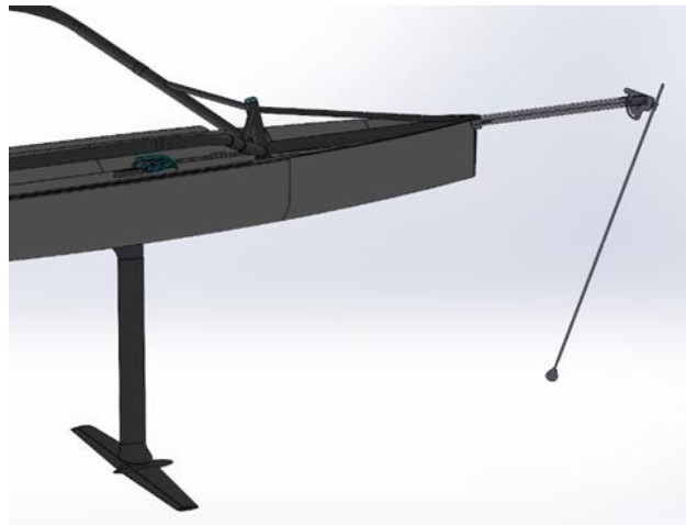
Figure 1-19: main foil control system overview
